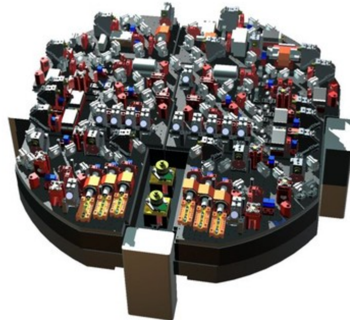
FIG. 2 (color). Mach-Zehnder interferometry of a BEC in microgravity as realized in the ZARM drop tower in Bremen (a) where absorption imaging (b) brings out the interference fringes (c). The preparatory experimental sequence (a) includes capturing cold atoms in a magneto-optical trap (MOT), loading an Ioffe-Pritchard trap, creating a BEC, and applying the DKC followed by the adiabatic rapid passage (ARP). The remaining time before the capture of the capsule at the bottom of the tower is used for AI and imaging of the atoms. The AMZI below the atom chip [top plane of (b)] is formed by scattering the BEC off moving Bragg gratings generated by two counter-propagating laser beams (red arrows directed along the y axis),
