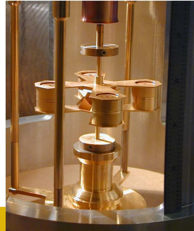
Microscope: French-German collaboration to test the WEP to 1 part in  $10^{15}$  using Ti-Pt test bodies and a Pt/Pt null comparison in a drag-free satellite operated in both inertial and rotating modes.
