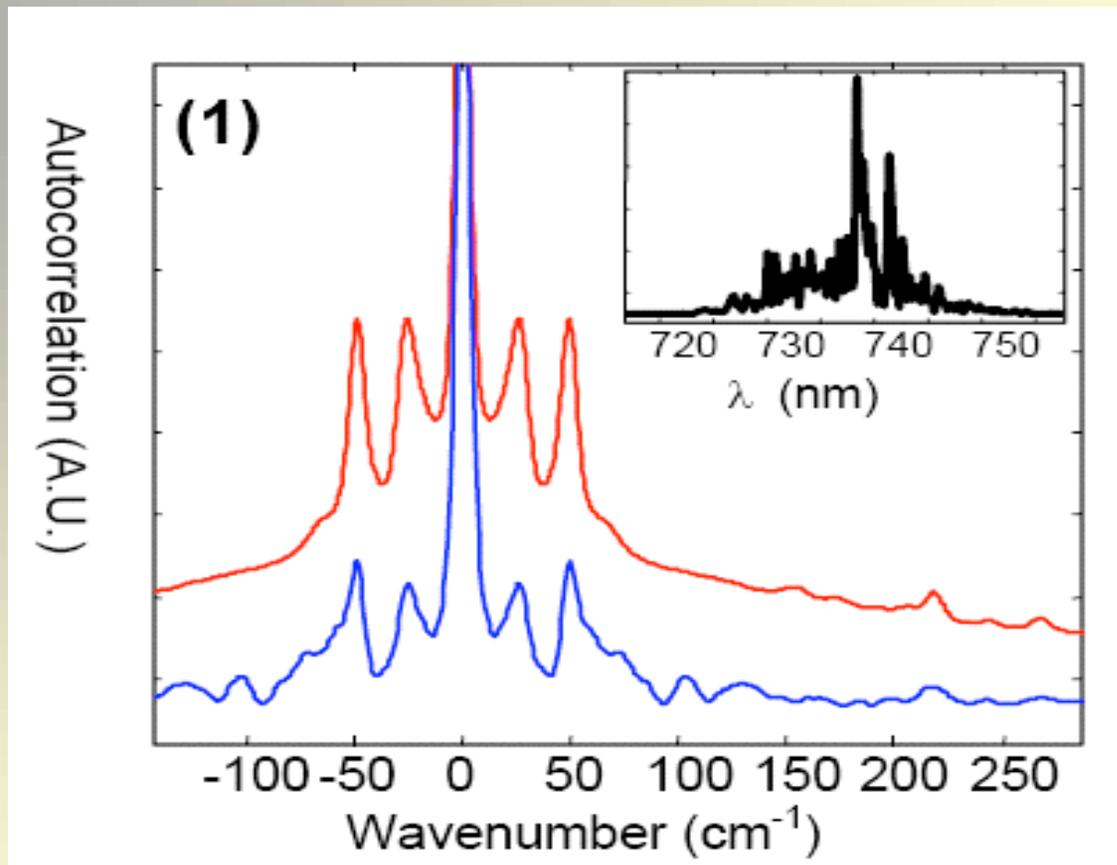
Experimental NASCARS spectrum of a mixture of toluene ( $782\text{cm}^{-1}$ ,  $1000\text{cm}^{-1}$ ,  $1027\text{cm}^{-1}$ ) with ortho-xylene ( $982\text{cm}^{-1}$ ,  $1049\text{cm}^{-1}$ ) mixture. Noise is introduced using spectral pulse shaper. Result is averaged over 100 noise realizations. Red curve is autocorrelation of Raman spectrum as reference
