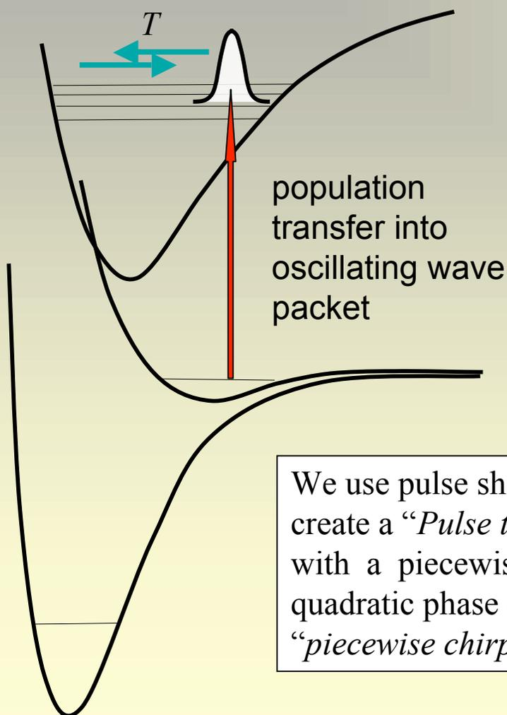
We use pulse shaping to create a "Pulse train" with a piecewise quadratic phase or a "piecewise chirp"
