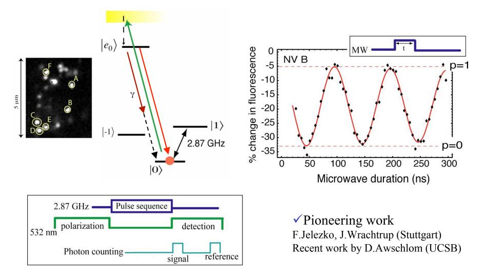
✓ Electron precession decay time (average over many runs):  $T_2^* \sim 1 \mu s$
