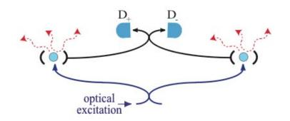
✓ Two centers create interferometer: photon detection creates remote electronic singlets!
