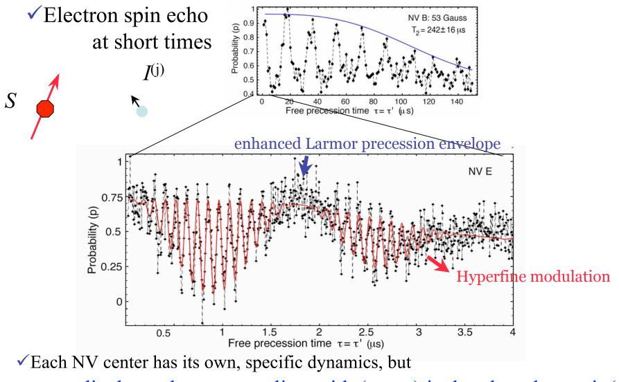
most display coherent coupling with (some) isolated nuclear spin(s)
