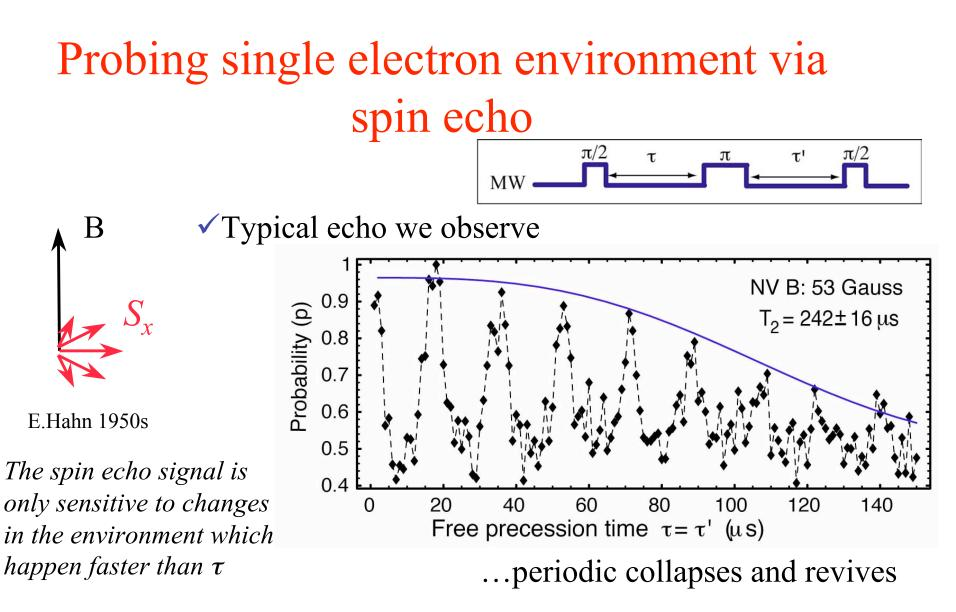
✓ Big effect:  $T_2 > 200 \ \mu s \sim 200 \ T_2^*$ : environment has long memory
