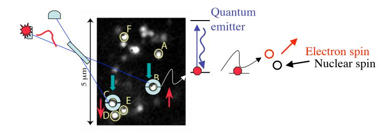
✓ Electron spin entanglement via photon scattering & single photon interference
