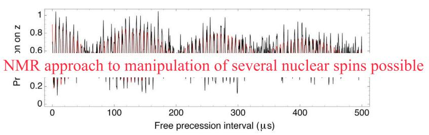
...modulated due to coherent interaction with another nuclear spin ( $I_2$ ),  $\checkmark$  Modulation rate controlled e.g. by B field orientation
