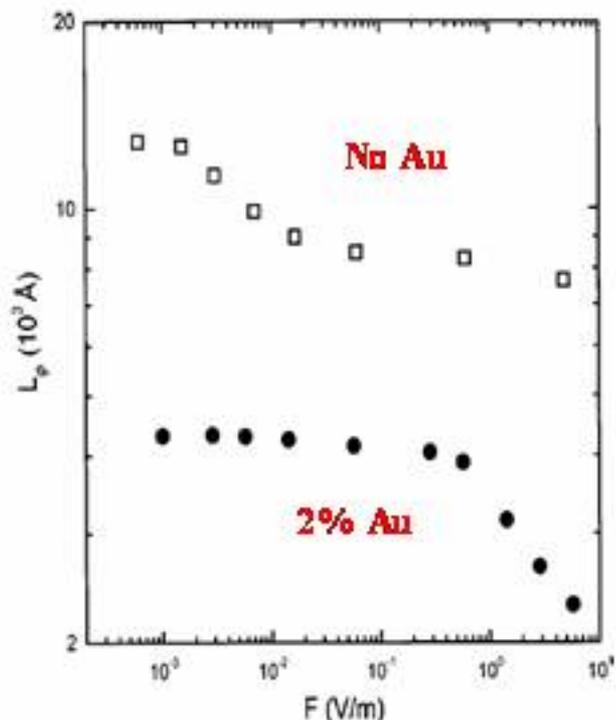
FIG. 9. The dependence of  $L_\phi$  on  $F$  for  $\text{In}_2\text{O}_{3-x}$  (sample No. 1) and  $\text{In}_2\text{O}_{3-x}:\text{Au}$  (sample No. 4).
