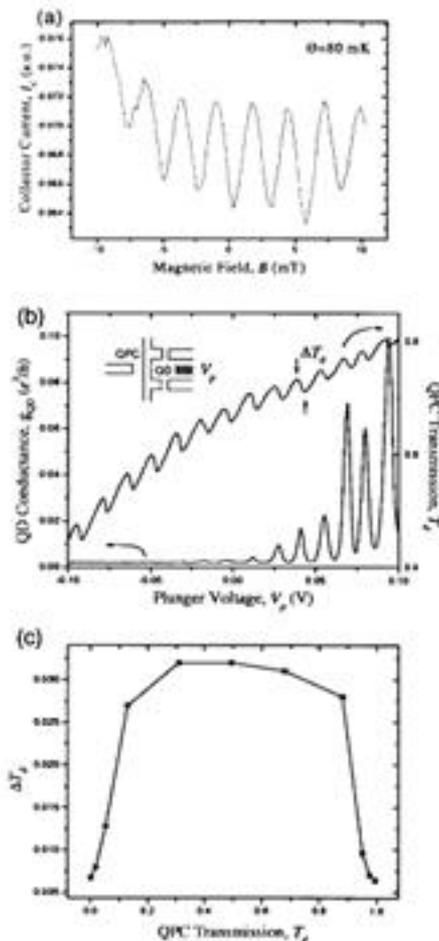
**Figure 2:** (a) AB oscillations in the collector current. (b) The conductance of the QD and that of the QPC detector as a function of the plunger gate voltage,  $V_p$ . The inset shows schematically the coupled structure. (c) The measured induced average change in the transmission probability of the QPC detector,  $\Delta T_d$ , due to charging the QD as a function of  $T_d$ .
