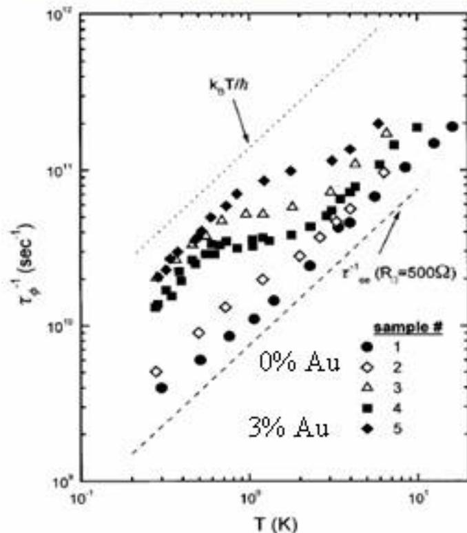
FIG. 11. Dephasing rates as a function of temperature for the studied films. These were obtained from the MR data at small  $F$  (typically  $6 \times 10^{-4}$  V/m at  $T = 0.28$  K,  $3 \times 10^{-3}$  V/m at 1 K, and 0.3 V/m at higher temperatures). For comparison, we include the electron-electron dephasing rate  $\tau_{ee}^{-1}$  expected of a 2D system with  $R_{\square} = 500 \Omega$  (based on Ref. 20).
