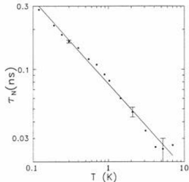
FIG. 2. Temperature dependence of  $\tau_N$ . The solid line is the best power-law fit  $\tau_N = 7.7 \times 10^{-11} (T/\text{K})^{-0.64}$ .
