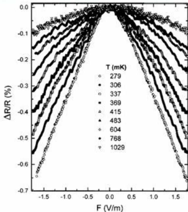
FIG. 12. Dependence of the differential resistance on  $F$  at several temperatures (sample No. 20).
