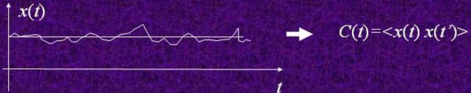
Classical measurement of a time-dependent quantity,  $x(t)$ , in a stationary state.
