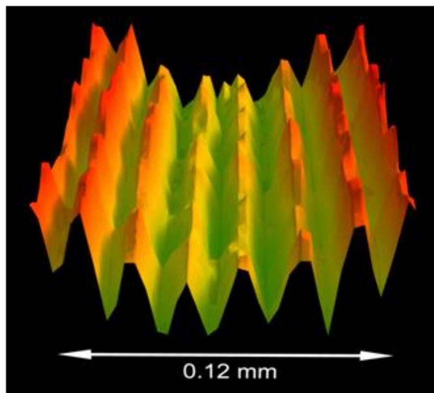
Interference of two expanding, overlapping BEC's,
