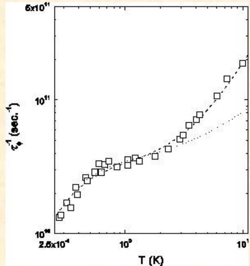
$1/\tau\phi$  vs  $T$  for the same sample. The dotted/dashed lines are fits to our theory with a symmetric well, using a reasonable prefactor and  $\Delta=3K$ , and adding the standard e-e AAK 2D/3D result.
