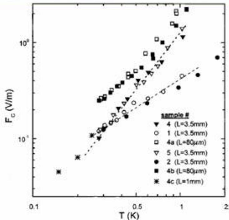
FIG. 14. The critical field (see text) for the various  $\text{In}_2\text{O}_{3-x}$  (circles) and  $\text{In}_2\text{O}_{3-x}:\text{Au}$  samples (other symbols) at various temperatures. Samples Nos. 4(a), 4(b), and 4(c) are from the same batch as sample No. 4 except that, for  $L$  is  $80\ \mu\text{m}$ , and for sample 4(c)  $L = 1\ \text{mm}$  (the latter was measured by D. Shahar). Dashed and dotted lines depict slopes of 1 and 2, respectively, as guides to the eye.
