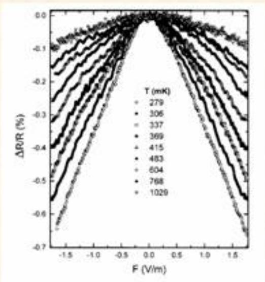
FIG. 12. Dependence of the differential resistance on  $F$  at several temperatures (sample No. 20).
