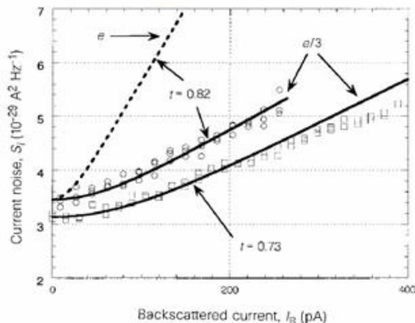
**Figure 3** Quantum shot noise as a function of the backscattered current,  $I_B$ , in the FQH regime at  $\nu = \frac{1}{3}$  for two different transmission coefficients through the QPC (circles and squares). The solid lines correspond to equation (2) with a charge  $Q = e/3$  and the appropriate  $t$ . For comparison the expected behaviour of the noise for  $Q = e$  and  $t = 0.82$  is shown by the broken line.
