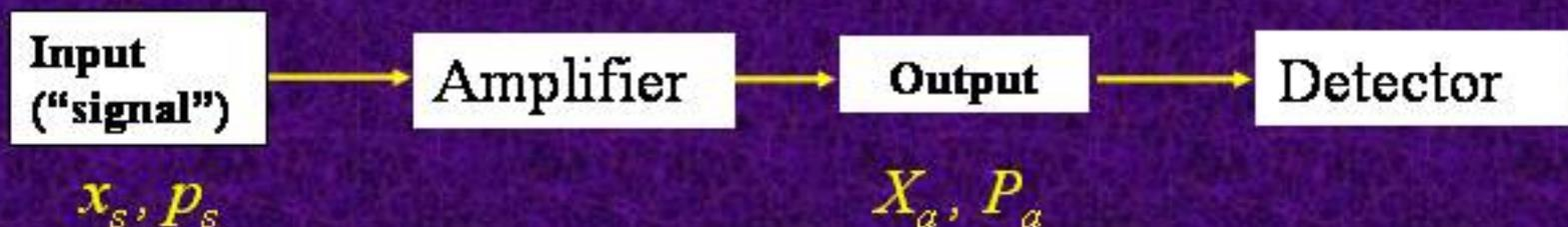
In order to keep the linear input-output relation, with a large gain, the amplifier must add noise
